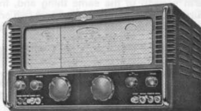
Eddystone 770U 6-band 15-valve double superhet 150-500 Mc/s
